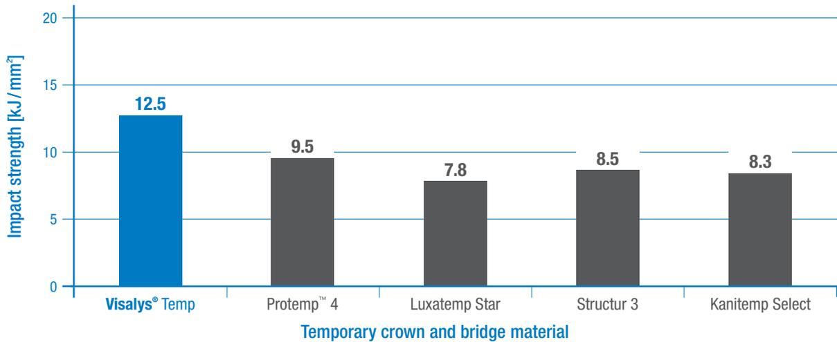
Measurements from the University of Erlangen, based on DIN EN ISO 179, DIN 53453
